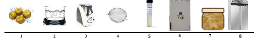
Figure 2. Sample preparation for PEF processing at laboratory scale. (1) Washing and cutting, (2) Pre-treatment, (3) Mash, (4) Refining, (5) Escherichia coli inoculation, (6) PEF pasteurization, (7) final product, (8) Refrigerated storage.
